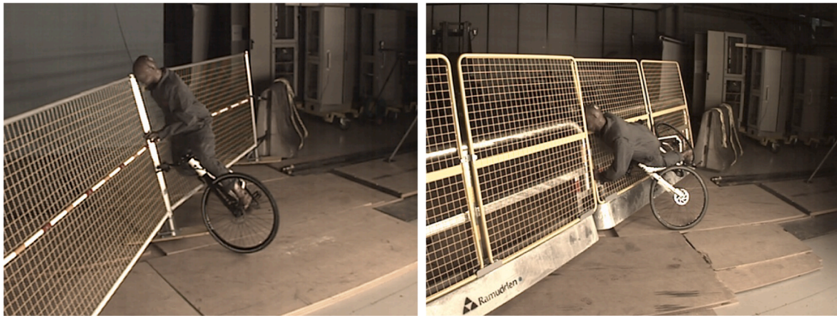
Fig. 7. Examples of cases when the head hit the railings of the fences.
