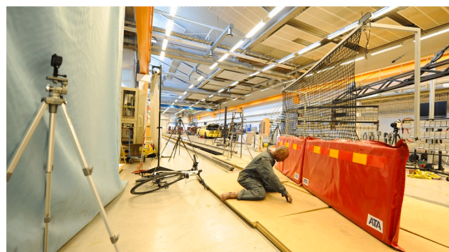
Fig. 10. The outcome of a 20-degree crash into REBLOC Concrete barrier with ATA Bicycle net without the fabric.
