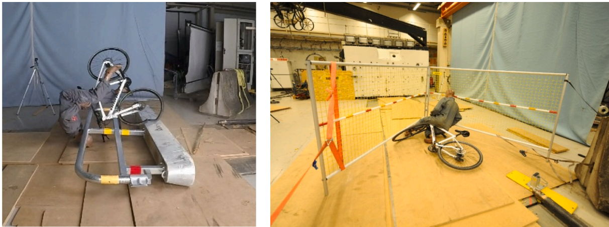
Fig. 5. A scenario with a straight crash into a single TA-barrier (at the left) and a Jonsered SafePass GC Barrier (at the right), both in 25 km/h.
