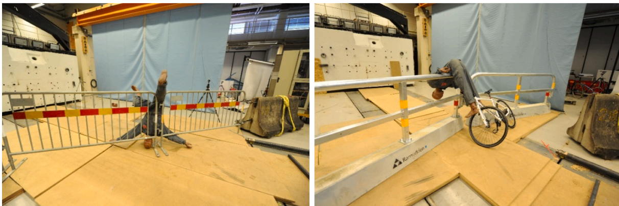
Fig. 3. The outcome of a 45-degree crash into Ramudden steel barrier (at the left) and a straight crash into a TA-barrier (at the right), both in 25 km/h.
