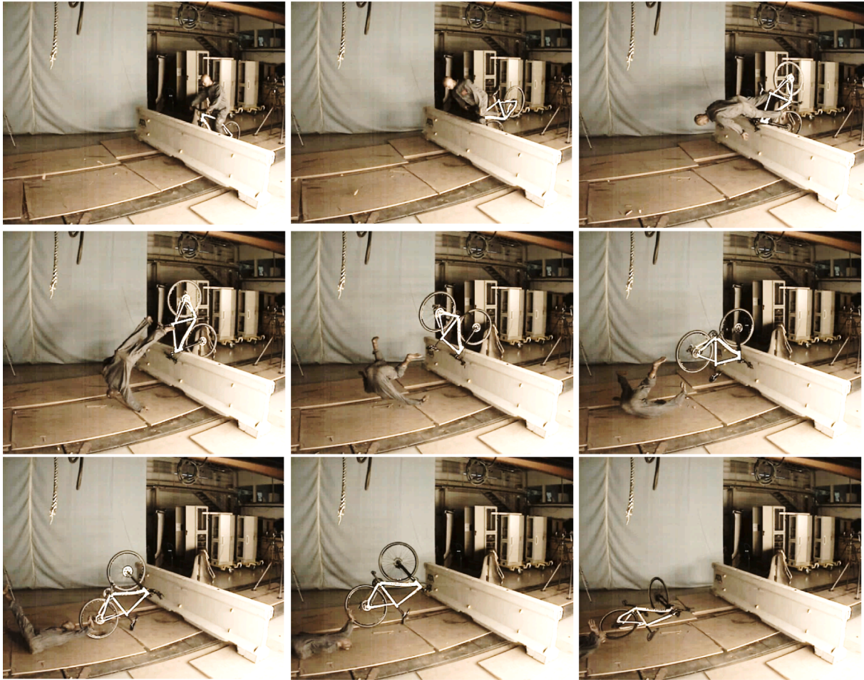
Fig. 2. A straight crash into a REBLOC Concrete barrier in 25 km/h, resulting in a somersault over the barrier for both “cyclist” (75 kg) and bicycle.
