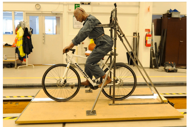
Fig. 1. Hybrid II 50th percentile crash test dummy on a bicycle mounted on the rig specially constructed for the purpose of performing simulated single-bicycle crashes.
