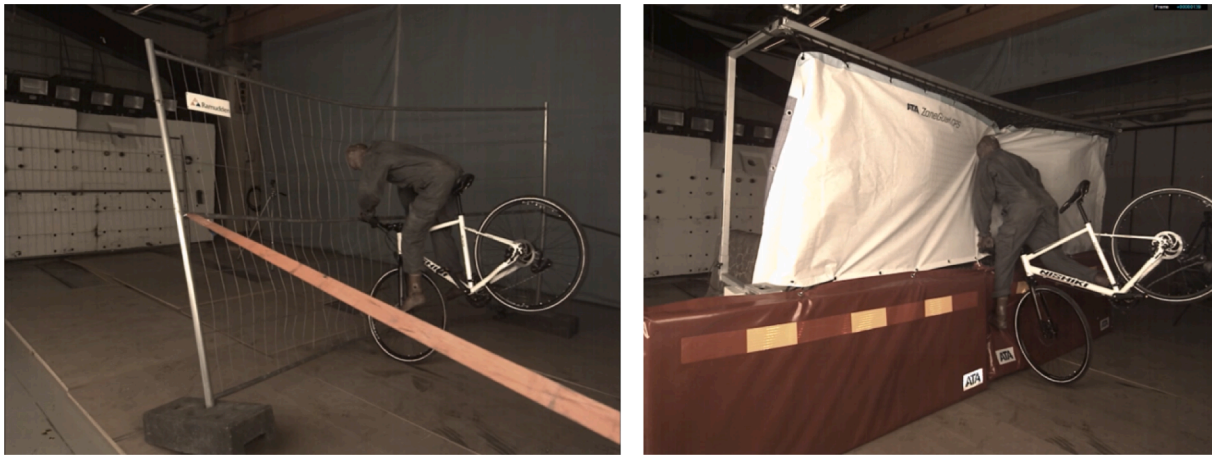
Fig. 4. To the left the crash dummy hits the head at impact with the construction fence. To the right the crash dummy's head hits a soft net with fabric that absorbs the energy from the impact.
