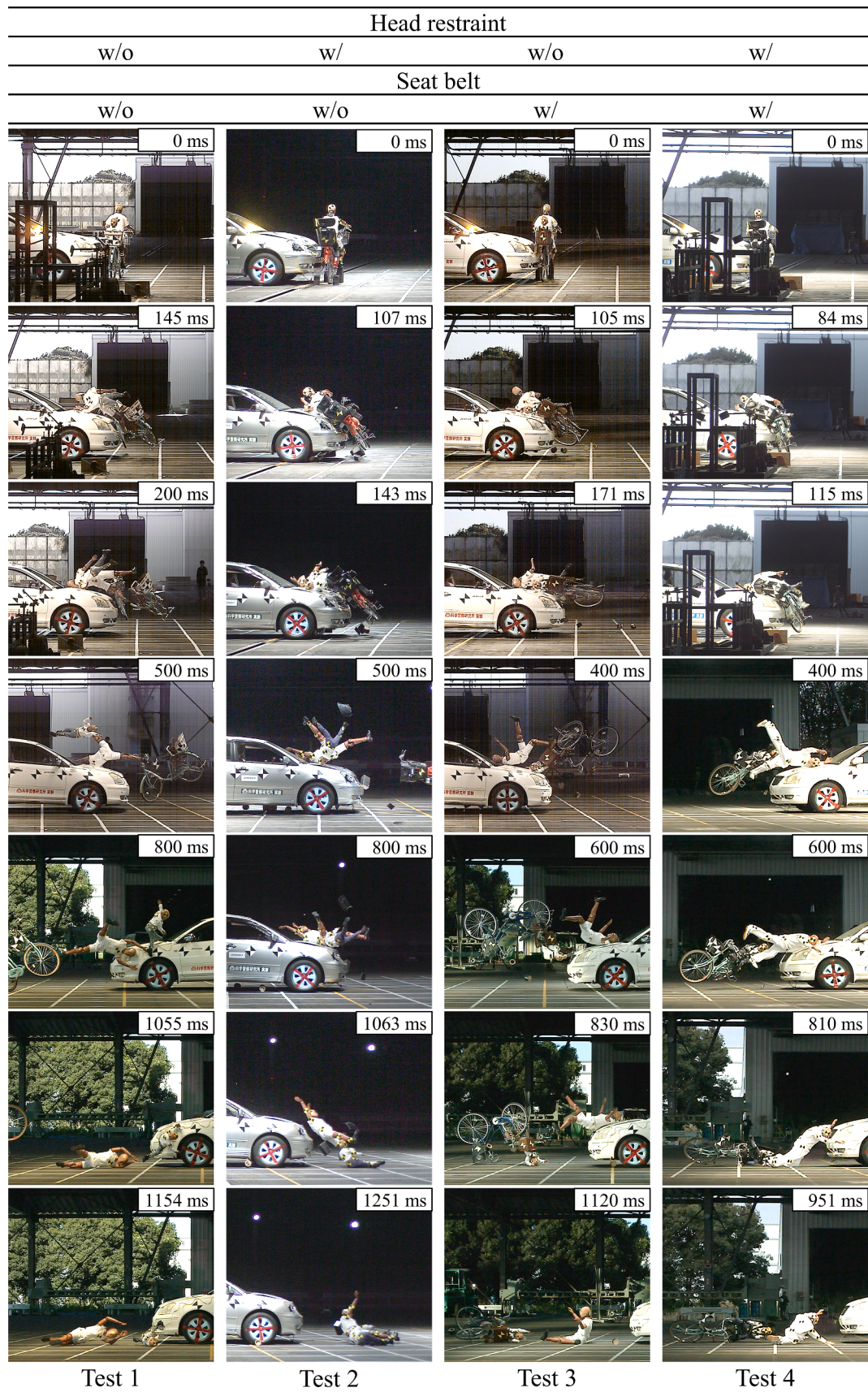
Fig. 6. Kinematic behaviors of the dummies and the bicycles in the collision tests.
