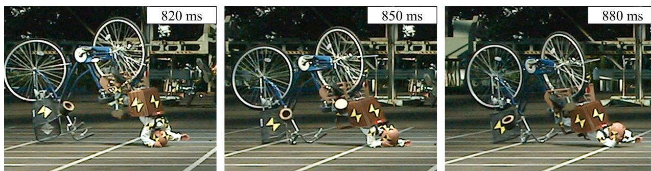
Fig. 9. Collision of the child dummy with the road surface in Test 3.
